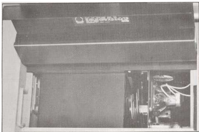
Lamp is readily accessible by lifting lamphouse cover. Press spring clip at end of socket base to release lamp assembly.
