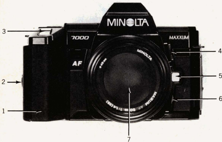
1. Soft grip. 2. Interchangeable battery holder. 3. Electronic shutter release. 4. Aperture setting keys. 5. Lens release. 6. Auto/manual focus switch. 7. 50mm f/1.4 auto-focus lens. 8. Shutter-speed setting keys. 9. Program reset switch. 10. On/off switch. 11. LCD display panel. 12. Rewind switch. 13. Dedicated hot shoe. 14. Drive selector. 15. ISO/ASA selector. 16. Auto compensation selector. 17. Exposure mode selector.
