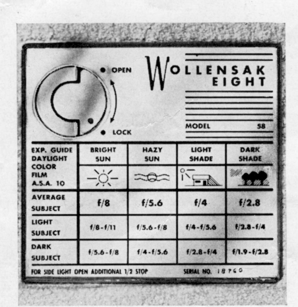
Your Wollensak "58" and "53" cameras have a convenient exposure guide mounted on the side of the camera. This guide has been computed for outdoor color film, rated ASA 10, and the normal camera speed of 16 frames per second.
