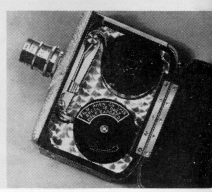
that the film is under the aperture plate flange. Swing the gate until it contacts the aperture plate flange. (Note: the gate is automatically held in closed position when the camera door is locked.) Pull the film through the gate, and, following the line with the arrow, around the lower guide post.
