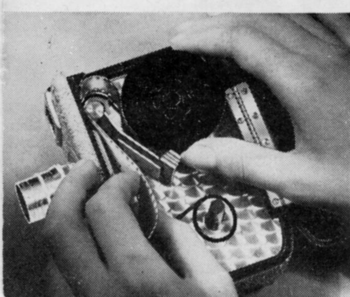
Set Footage Meter to "RED DOT" (loading position) before loading film.
