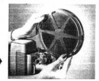
Seat full reel of film on UPPER SPINDLE with the square hole of reel towards the hub of the spindle. Properly spooled film should unwind from the front of the reel with dull (emulsion side) of film toward screen.
