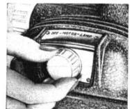
Turn MOTOR-LAMP SWITCH to right until two clicks are felt. First click position starts blower . . . second turns on lamp.
