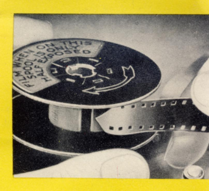
Run off 1 or 2 inches of film by pushing starting button down momentarily, at the same time, holding film gate closed.
