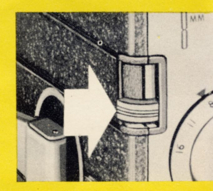
Pushing the starting button *up* takes a single picture at a time. This is called "single-frame exposure." Ask your dealer for a free copy of "Tips on Movie Making Tricks" booklet for further information on use of single-frame exposure.
