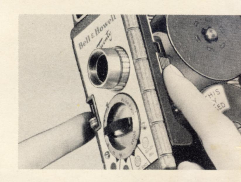
Push starting button down and run film until footage counter indicator reads 0.
