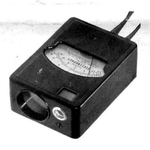
The increasing use of Kodachrome Film demands an exposure meter to use with this film in the simplest possible way. The new ELECTROPHOT fully meets this demand. Point the meter at the scene to be taken and read the Red Scale. Nothing could be simpler. In all ELECTROPHOT models it has been our aim to supply a meter easy, quick and convenient to use and this policy has been followed in producing this model.
