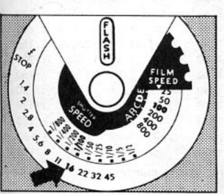
step 3: Proceed as for range finding. When subject's face\* is correctly framed the range may be read at the top of the slide, and the proper f/stops and shutter speeds will be found opposite each other on the two black dials. For shutter speed slower than 1/50 of a second, use f/stop opposite 1/50.
