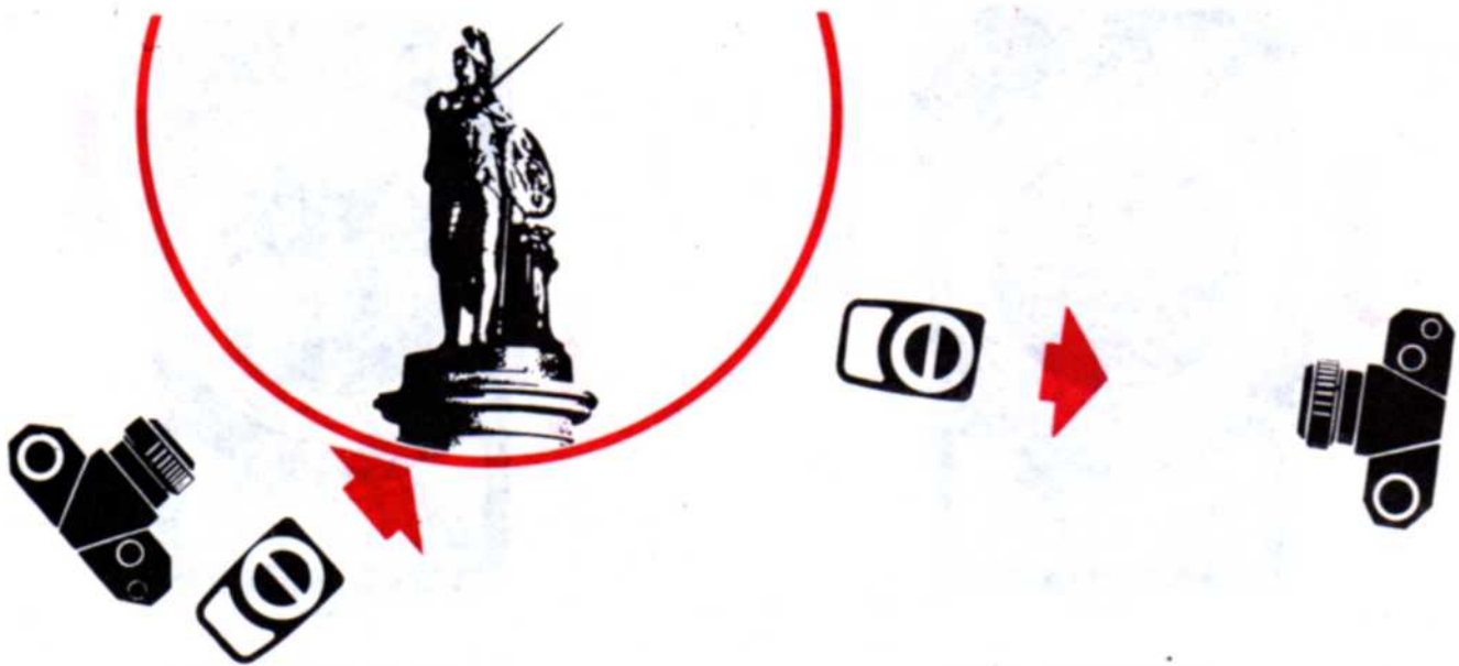
Determination of shutter speed or lens aperture by incident light method
