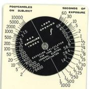
PLACE LIGHT METER AT SUBJECT. POINT LIGHT CELL HALF WAY BETWEEN LIGHT SOURCE AND CAMERA. READ FOOTCANDLES AT IMPORTANT POINTS OF SUBJECT. THEN SET AVERAGE FTC. OPPOSITE EXPOSURE INDEX. FOR COLOR FILM, FTC. RANGE SHOULD BE 4 TO 1 OR LESS.
