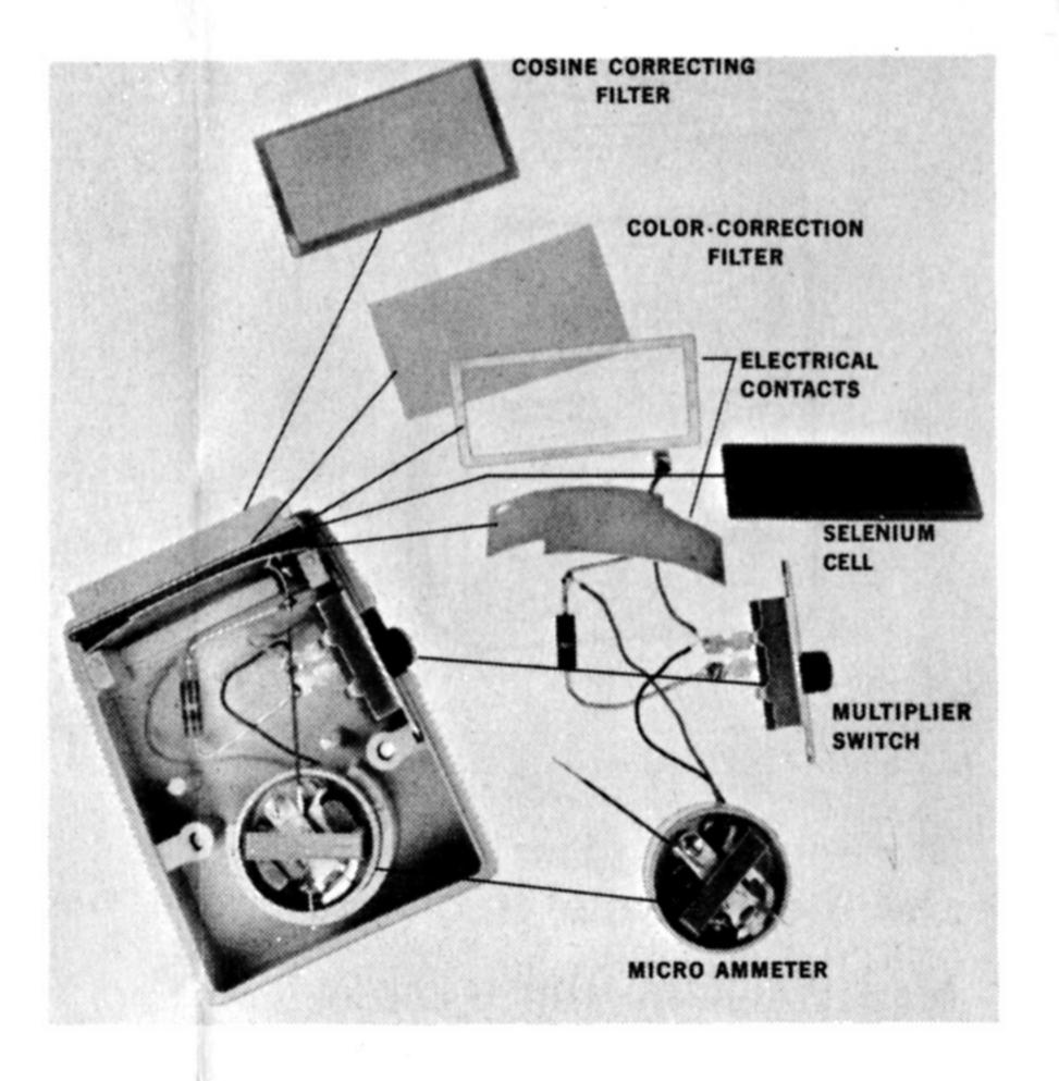
The General Electric Type 213 Light Meter is a pocketsize, color- and cosinecorrected light indicating device capable of reading to 500 footcandles on its basic scale and to 5000 footcandles with the use of a built-in multiplying switch.
