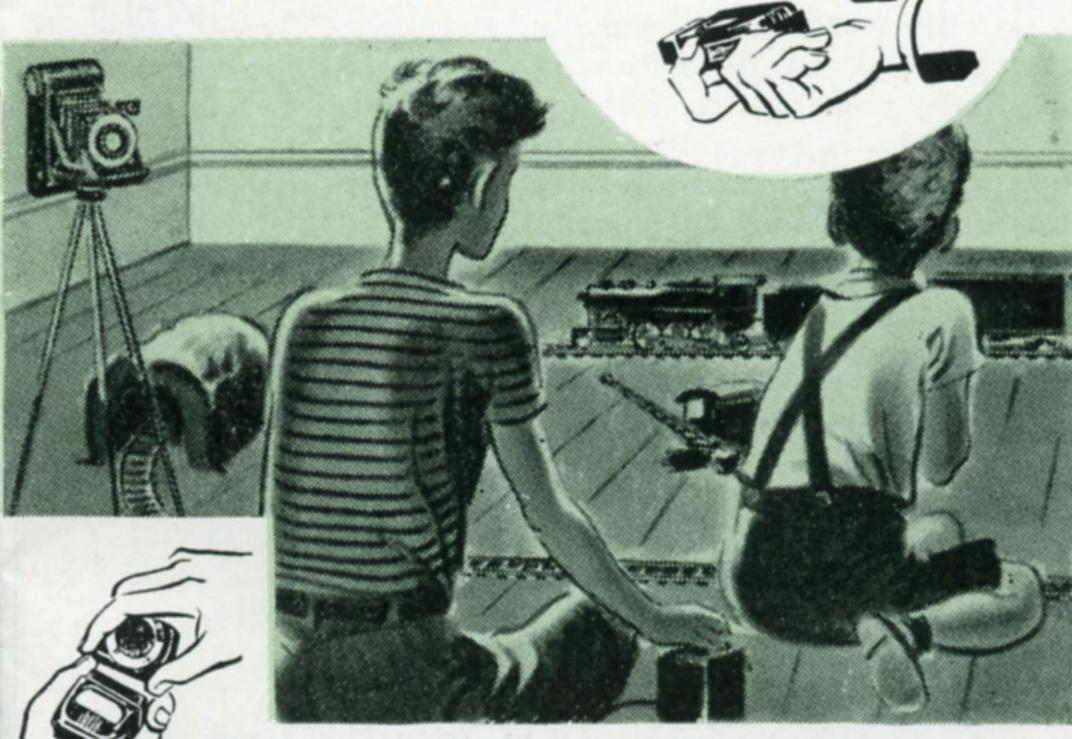
When no reading is obtained with hood on, remove the hood (by bending toward you) and point the meter at the camera, from the subject, and read light value indicated.
