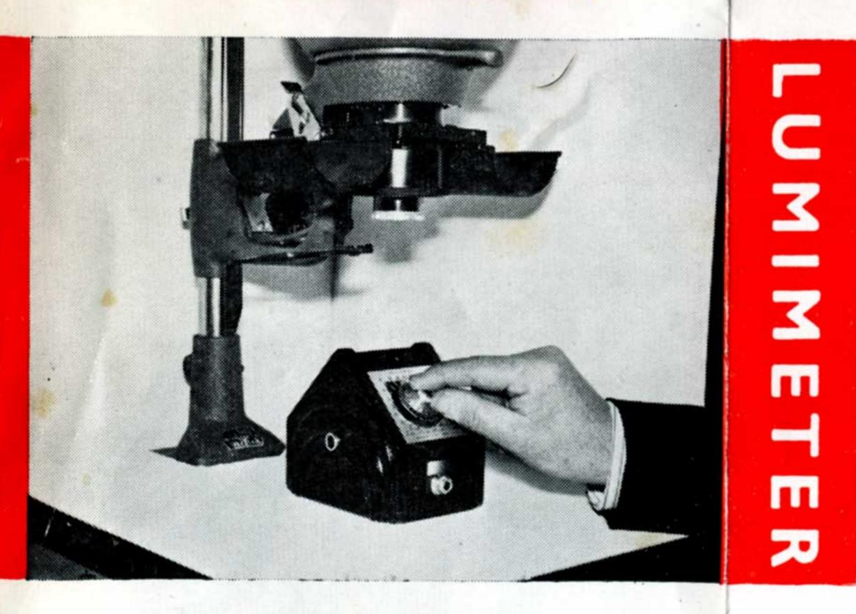
When using the Lumimeter for the first time it is necessary to adjust it to suit your enlarging equipment. This adjustment is quite simple and automatically takes into account such things as electricity supply voltage, type of enlarger lamp and development technique. Before you can adjust the Lumimeter however, you must be familiar with its use, so start by taking a reading on an average negative.
