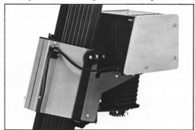
Move the lifting lever arm so that the lifting lever mounting screw is approximately centered in the oval cut-out in the arm, and tighten the screw. This adjustment controls the amount of lamphouse lift, and can be changed as desired.
