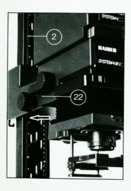
The Column (2) is provided with various scales – in cm and inches – also indicating the magnification factors for 90, 80 and 55 mm lenses. All dials and markings are referenced to the lower edge of the Head Mounting Bracket (22).
