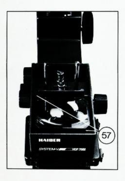
Release the two fastening screws (57), and lift out the double condensor. Reverse the procedure to insert a condensor. Return the lamp head.
