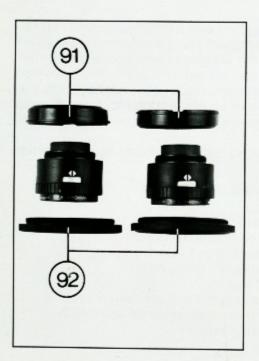
The lens is mounted with the help of two lens adapter rings (91) and (92). First unscrew the centering ring (92) in the lens panel (82), and take the lens adapter ring (91) out of the centering ring (92).
