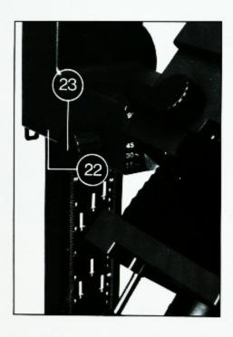
To tilt the enlarger head, release the clamping screw (23), tilt the head in the manner required; firmly retighten the clamping screw. Marks on the face side of the supporting arm (22) become visible when the enlarger head is tilted. These marks indicate the inclination angle of the enlarger head in relation to the horizontal.
