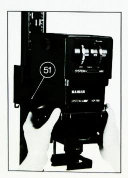
Rotation of the swivel grip (51) lifts the upper section of the enlarger head, simultaneously partly opening the compound negative carrier. The film strip can now be inserted from the front with its emulsion side facing downwards. Precise adjustment is achieved when the film strip comes up against the correspondingly adjusted stop ins (63). The swivel grip (51) is now turned back, thus reclosing the compound negative carrier. The procedure is repeated to advance the film.
