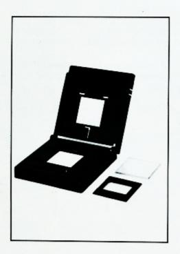
The VP 3502 enlarger is equipped with a small-picture format negative holder with an AN glass upper insert and format lower insert (picture left). After removing the AN glass insert above and the format insert below, slides can be inserted directly into the lower part of the negative holder. This negative holder does not have adjustable masking strips. The unit can be re-equipped for formats up to 6 x 7 mm with the negative holder described as well.
