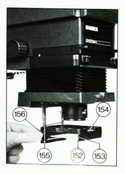
The below-lens filter holder has two insert slots (152) for square filters of between and 67 mm width, and another insert slot (153) in the center for masks up to 1 mm thickness. Frames filters to process variable-contrast papers can be inserted in a special holder (154) at the top of the filter carrier (151).
