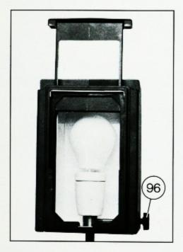
To replace and exchange the opal lamp in a B & W head it is necessary to lift the lamp head off the condensor housing (5). First of all disconnect the mains plug. The lamp can be screwed in after the filter drawer (39) has been removed.
