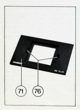
The 4489 size insert (71) must be placed in the lower part of the compound negative carrier when enlarging framed slides with an overall size of 5 x 5 cm. This insert is provided with grip recesses (76) so that the slides can be more easily removed.
