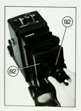
The lens with the screwed on adapter ring is now inserted from above into the centering ring (92), which, in turn, is screwed into the lens panel (82). Ensure that the f-stop values of the lens are facing to the front.
