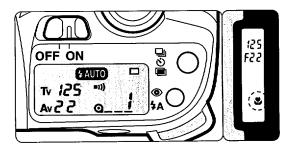
This mode is useful for close-up photography. This mode favors smaller apertures to maximize the depth of field, ensuring sharp focus of a close-up subject.
