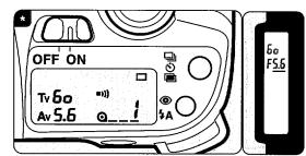
\* When the shutter release button is depressed halfway down, the shutter speed and aperture value will be displayed in the viewfinder and on the LCD panel. The bar underneath the aperture value indicates that you can change the aperture setting.
