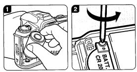
Replace the battery when the data information on a picture or the LCD panel becomes weak or invisible. The battery will last for approximately 3 years. The data back uses one 3V lithium battery, type CR2025.
