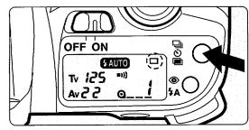
Depress the drive button until [□] appears on the LCD panel.
