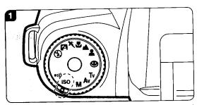
This camera automatically reads the film speed from the film's DX code. However, the film speed setting can be changed. If you use a non-DX coded film, set the film speed manually.
