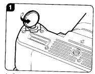
Open the battery chamber cover by using a coin, etc. as shown in the illustration.
