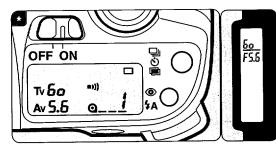
\* When the shutter release button is depressed halfway down, the shutter speed and aperture value will be displayed in the viewfinder and on the LCD panel. The bar underneath the shutter speed indicates that you can change the shutter speed.
