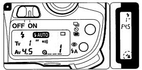
\* When the shutter release button is depressed halfway down, [🔩] is displayed in the viewfinder. The shutter speed and aperture setting are also displayed in the viewfinder and on the LCD panel.
