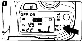
At each press of the flash mode button, the flash mode on the LCD panel switches as shown in the chart.
