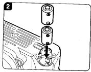
Load two 3V lithium batteries (CR2) or equivalent as shown in the illustration.
