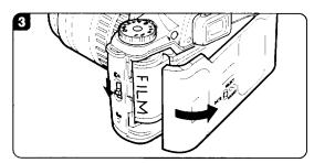
3. Open the back cover and remove the film.
