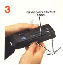
**OPEN** the FILM-COMPARTMENT DOOR by depressing the LATCH and lowering the door.
