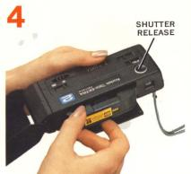
INSERT a film cartridge into the camera. Close the door until it locks with the camera body.
