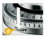
When you have set the light value, for instance 10, you can read off one of the following aperture-speed combinations against the triangle \( \Delta\) index mark (9):
